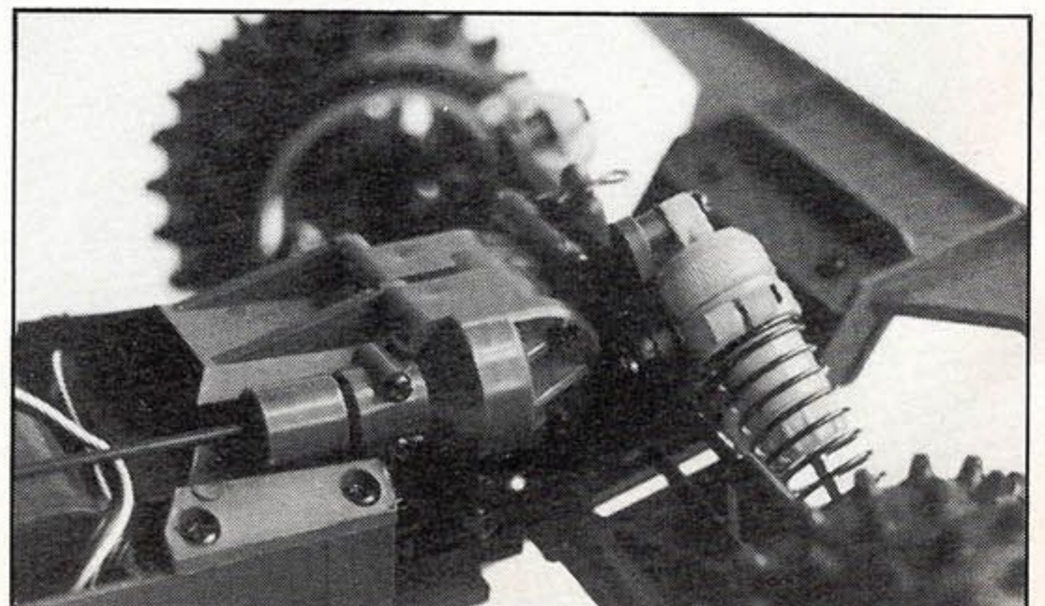
Front differential with shaft drive, collar needs to be secured during construction (see text).
