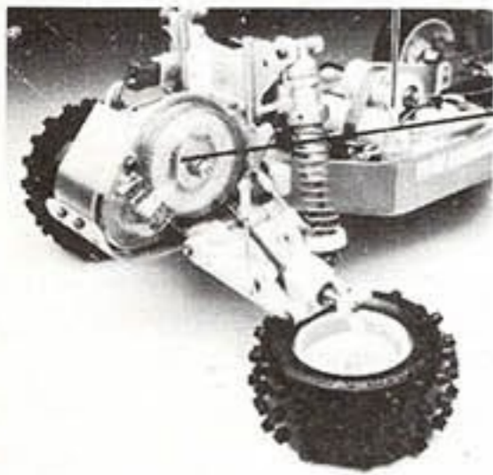
Sealed gearbox VariLok differential
